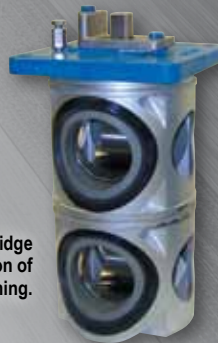
A double sealing system on the upper and lower stems guards against any possible leakage. If service becomes necessary, just remove four bolts and the cartridge slides right out the top of the strainer body.
